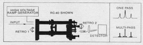
Another type of application is to operate two spectrographs in series. One particular application uses a grating spectrograph and a Fabry-Perot. The series operation allows the high resolution of the Fabry-
