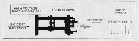
Filtering: The Fabry-Perot in a static mode will transmit a plane wavefront traveling normal to the interferometer axis if the wavelength is within the bandpass of the interferometer.
